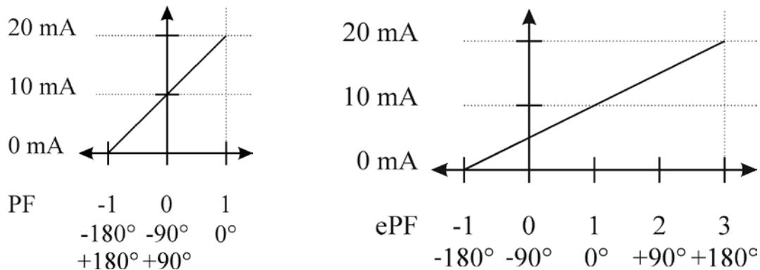
The power angle represents the angle between the first voltage harmonic and the first current harmonic for each individual phase. The total power angle is calculated from the total active and reactive power (see equations for total power angle, in chapter 8, "Appendix B: Calculations and equations on page 47). A positive sign shows inductive load, and a negative sign shows capacitive load.
